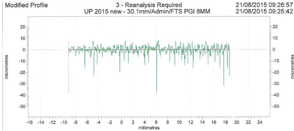
Figure 5 – Surface roughness of the new spiral
