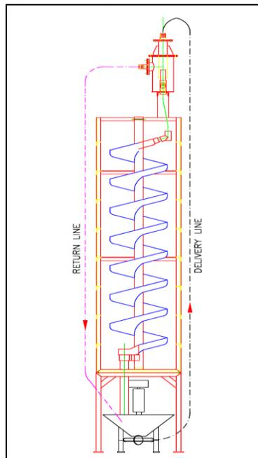
Figure 2 - Spiral test rig setup
